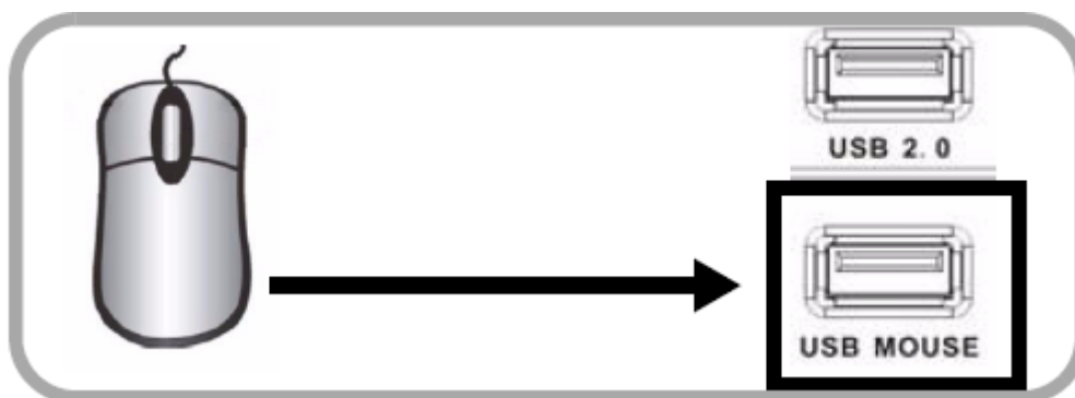
Figure 1.0 Connect a USB mouse to the bottom USB port on the front panel
