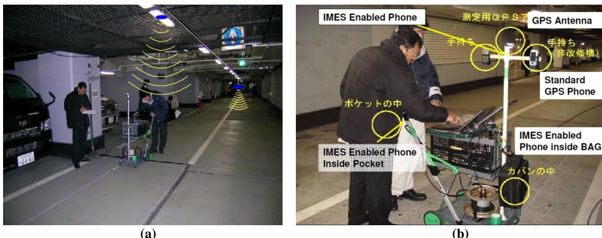
Figure 8: Indoor demonstration of IMES at an underground parking area. (Source: Manandhar et al. (2008))
