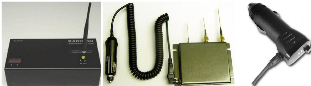
Figure 3: GNSS jammers found during casual browsing of the internet. The sources of the figures are not given for obvious reasons. Readers are reminded that GNSS jamming is illegal.
