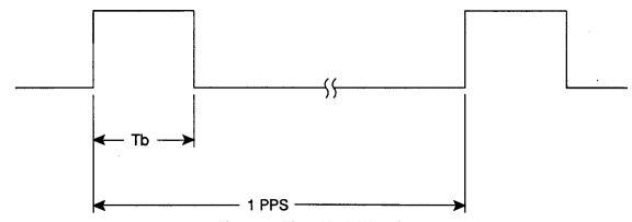
Figure 7: Time Mark Waveform
