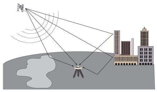
Figure 28: Illustration of GPS Signal Multipath
