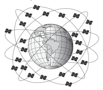
Figure 24: NAVSTAR Satellite Orbit Arrangement
