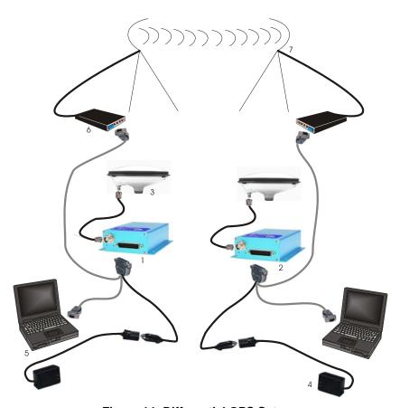
Figure 14: Differential GPS Setup
