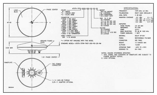
Figure 16: GPS Antenna 201-990147-606 (+26 dB)
