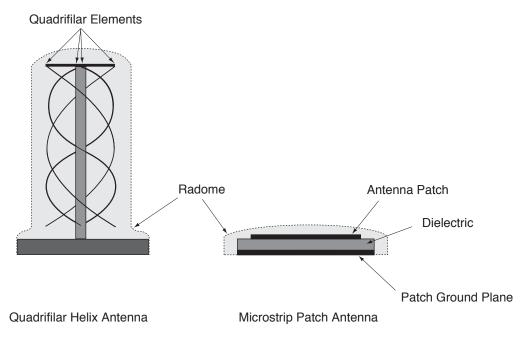
Figure 30: Illustration of Quadrifilar vs. Microstrip Patch Antennas
