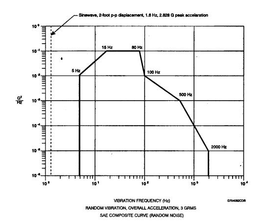
Figure 12: SAE Composite Curve (Random Vibration)
