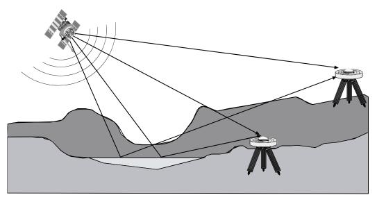
Figure 29: GPS Signal Multipath vs. Increased Antenna Height
