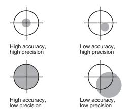
Figure 26: Accuracy versus Precision<sup>1</sup>
