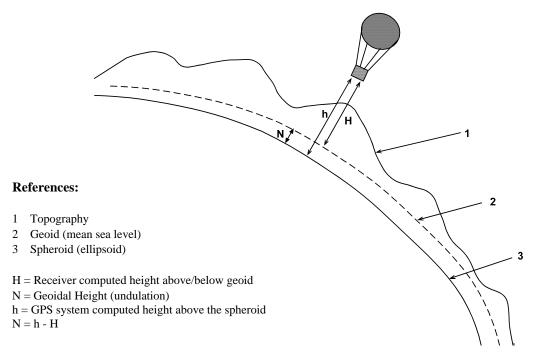
Figure 25: Illustration of Receiver Height Measurements
