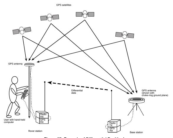
Figure 27: Example of Differential Positioning
