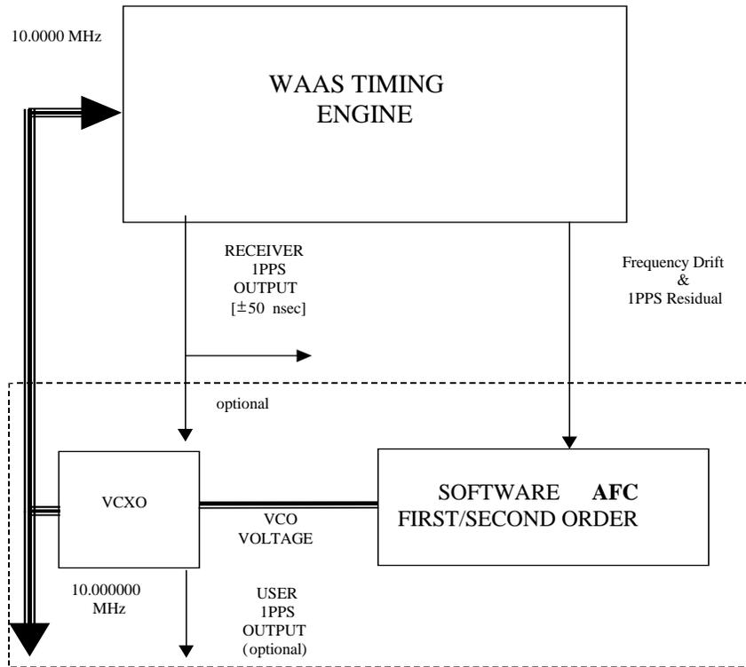
**Figure 3: One-Shot Alignment Mode Configuration**
