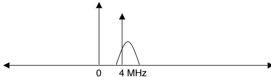
Because of the doppler shift, the reconstructed carrier is shifted in frequency. We reconstitute a frequency of  $F_{nom} + F_{doppler}$
