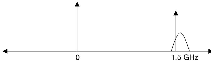
**Figure 5: Demodulated GPS Data (Doppler Present)**
