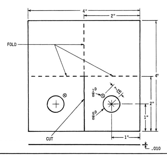
VAT-40 SERIES VOLT-AMPERE TESTERS DATE CODED "28" OR LATER WILL INCORPORATE THIS SHIELD.
