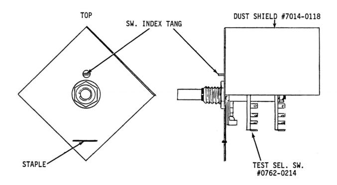
THE ADDITION OF THIS 'SWITCH' DUST SHIELD SUN PART No. 7014-0118 IS DESIGNED TO INCREASE THE RELIABILITY OF ALL VAT-40 VOLT AMPERE TESTERS BY SHIELDING THE TEST SELECTOR SWITCH ON THE TOP SIDE FROM DUST AND CARBON PARTICLES FROM THE CARBON PILE.
