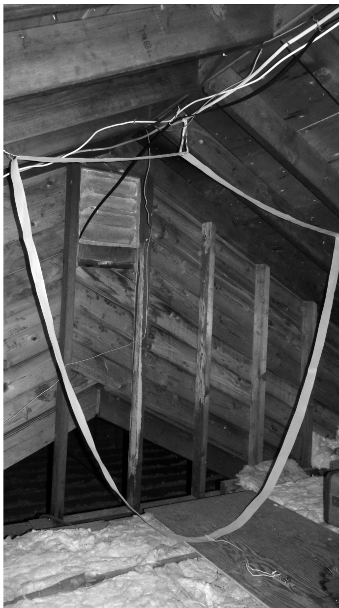
Figure 6 — The author's attic-mounted loop antenna. With the plane of the loop aligned toward Fort Collins, Colorado, the WWVB horizontally polarized H-Field cuts through the center of the loop and induces a voltage across it. The frequency standard amplifies and processes this signal.
