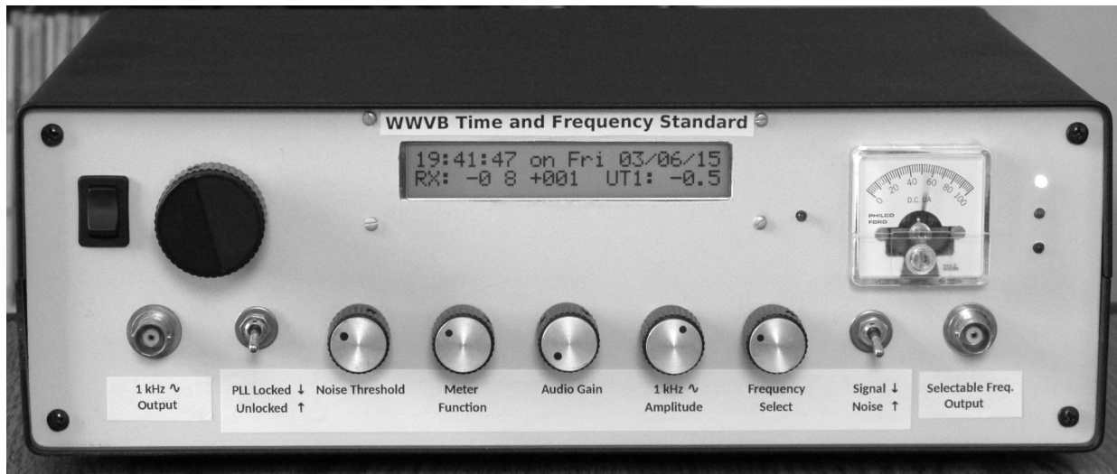
Figure 20 — Front view of the frequency standard in operation. The large knob on the upper left permits manual fine tuning of the VCTCXO, while the display provides the UTC date and time.
